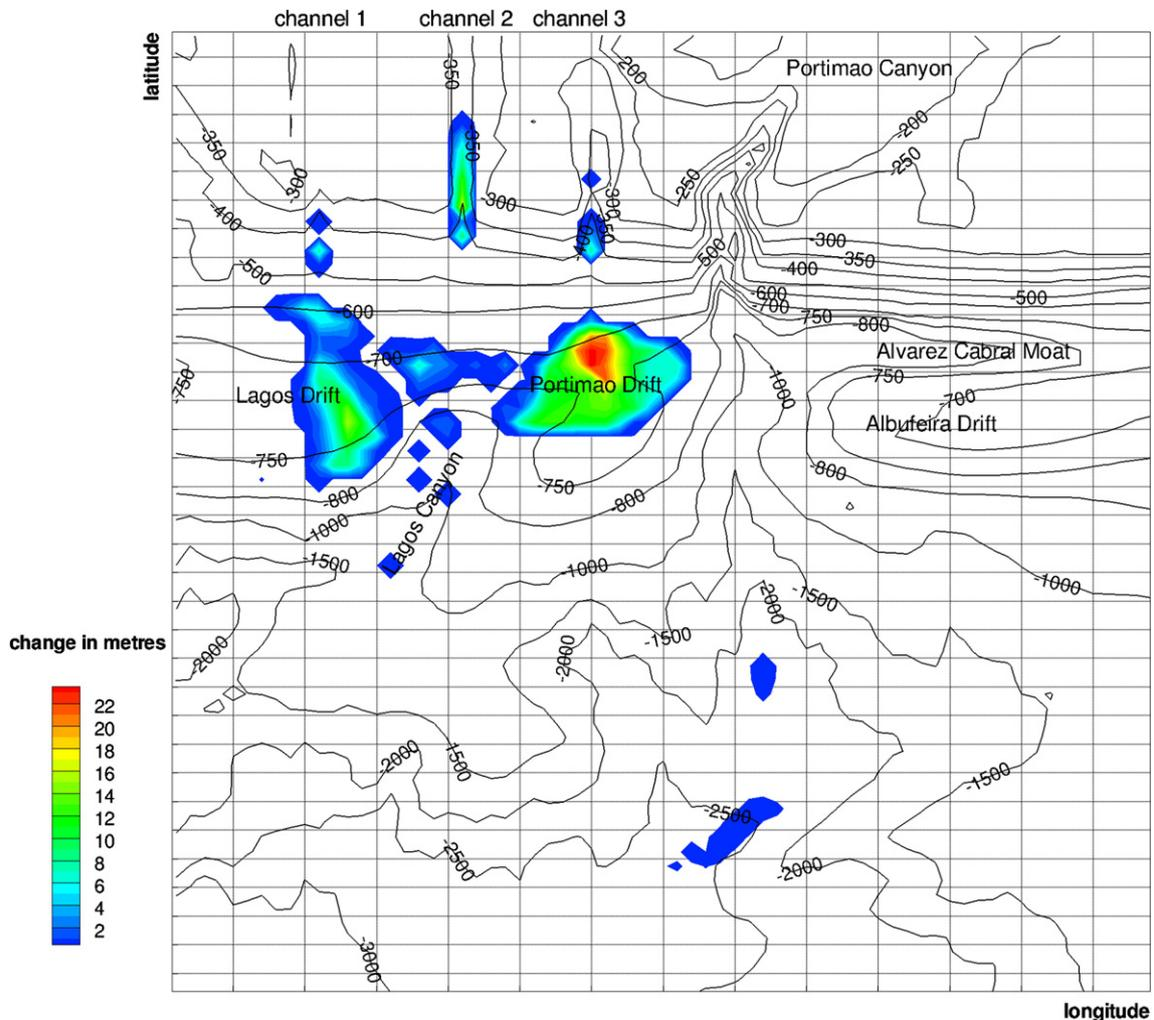
Fig. 8. Deposit thickness due to paleo-channel activity between 130 and 135 ka BP.
