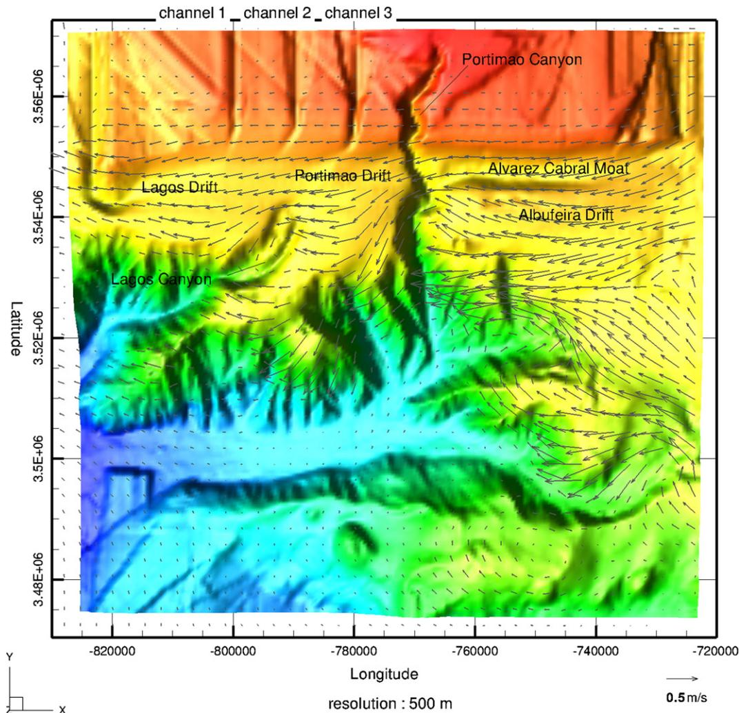
Fig. 2. 2005 MUW annual mean bottom velocities computed with the numerical model from Serra et al. (2005).
