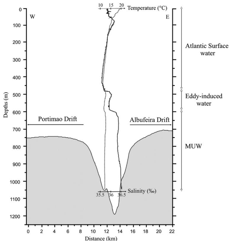
Fig. 8. Salinity (black line) and temperature (black broken line) depth-profiles from CTD.
