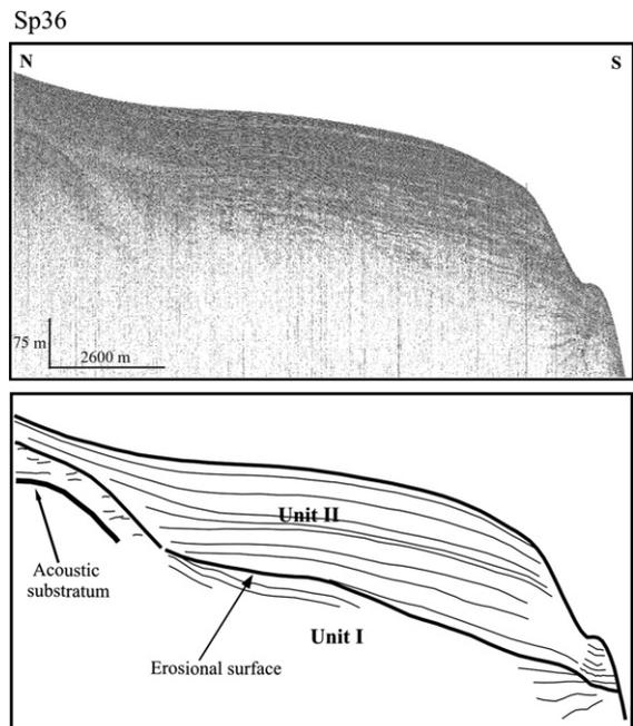
Fig. 7. Sparker seismic profile SP36 crossing Lagos Drift and its interpretation.
