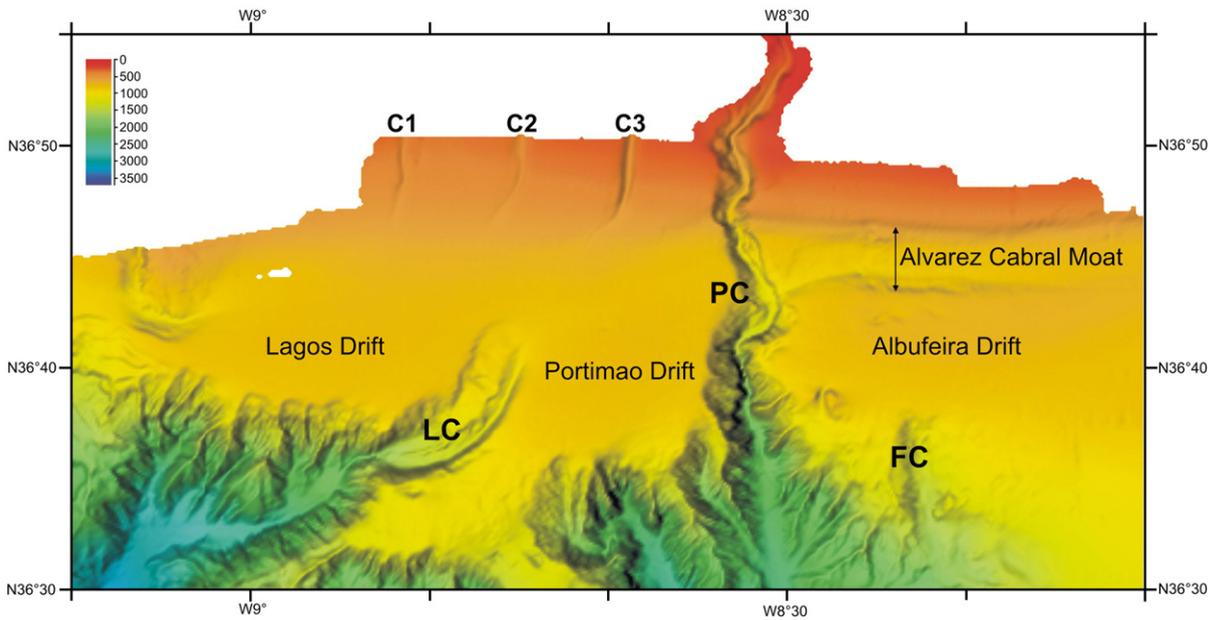
Fig. 4. 3D bathymetry showing the main morphologic features of the study area (PC: Portimão Canyon; LC: Lagos Canyon; FC: Faro Canyon; and C1, C2 and C3: Channels 1, 2 and 3).
