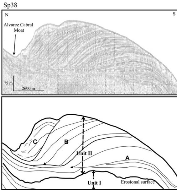
Fig. 6. Sparker seismic profile SP38 crossing Albufera Drift and its interpretation (see text for signification of sub-unit A, B and C).
